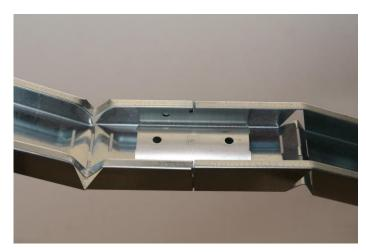
• connect the CONCAV & CONVEX Curving Studs to the primary metal framework with channel hangers, with an interaxle spacing of 30 cm (or 40 cm, depending on the radius of the curvature)
